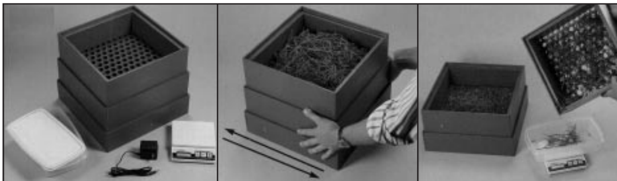
Figure 2 : Forage particle separator developed by Pennsylvania State University and available from: Nasco, 4825 Stoddard Road, Modesto CA 95356-9318, (209)545-1600. Price quoted in the 1996 Nasco catalog was US$195.
